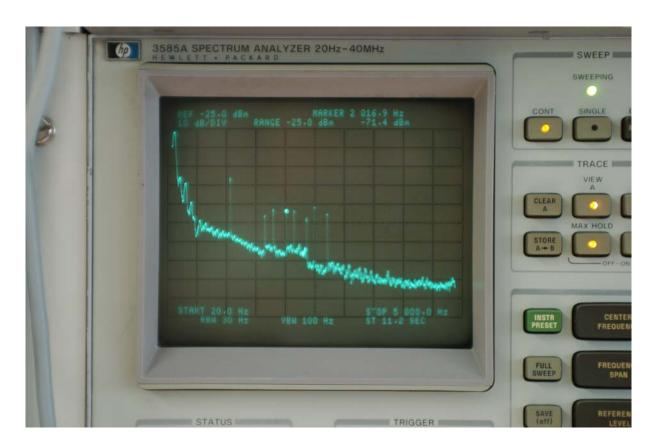
Here you see in comparison the same measurements of the Furutech RD-2. The complete area underneath the trace is much smaller, which means simply less energy dissipated. Also clearly can be seen the spikes of the harmonics of the 50 Hz signal (second and third peak from the left) Also some spikes of intermodulation can be seen on the right.
