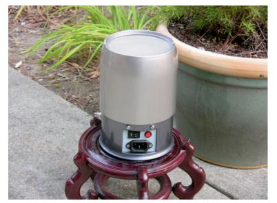
one play because of the CD player itself. Even though the effects of the RD-3 will last over 6 months it is ideally recommended that you demagnetize your disc before each playing. Also remember that you should only demagnetize 10 discs at a time and then wait 15 minutes to allow it to cool down between treating sets of 10 discs.
